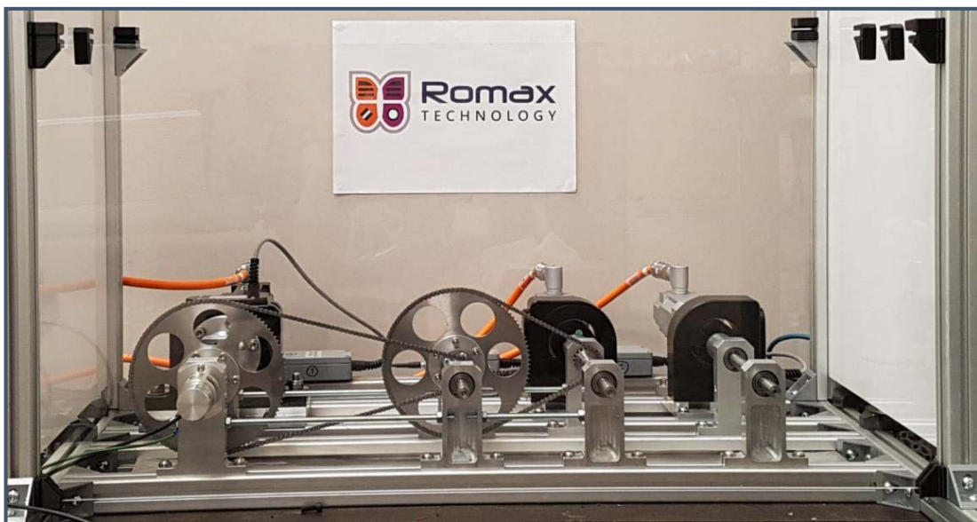
Figure 3: 1/25 scale PTO Test Rig at Romax Testing Facility
