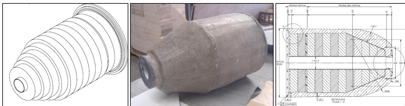
Figure 4: Manufacture of the fibreglass bullnose is similar to that of the TLA buoy. Profiled Divinycell sheet make up the rough shape which is then over moulded with fibreglass before being machined down to an accurate profile.
