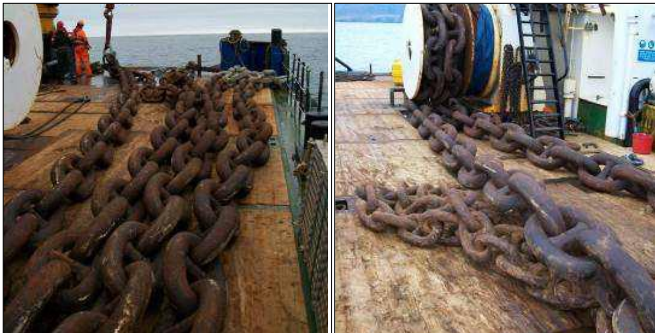
Figure 6: Mooring chain during deployment
