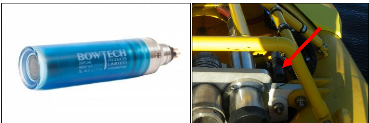
Figure 20: Bowtech Dive-cam used by PWP to give visual feedback of the latching process. These were installed on the protection frame on the end of the yoke (right).
