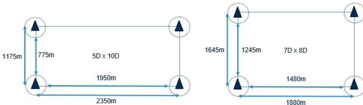
**Figure 7-2 Indicative layouts for WTG locations with more and less unidirectional wind resource.**
