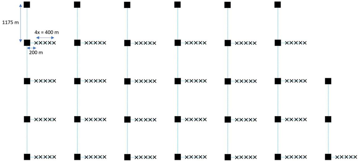
Figure 3-9: WTG and WEC layout (Scenario 14)
