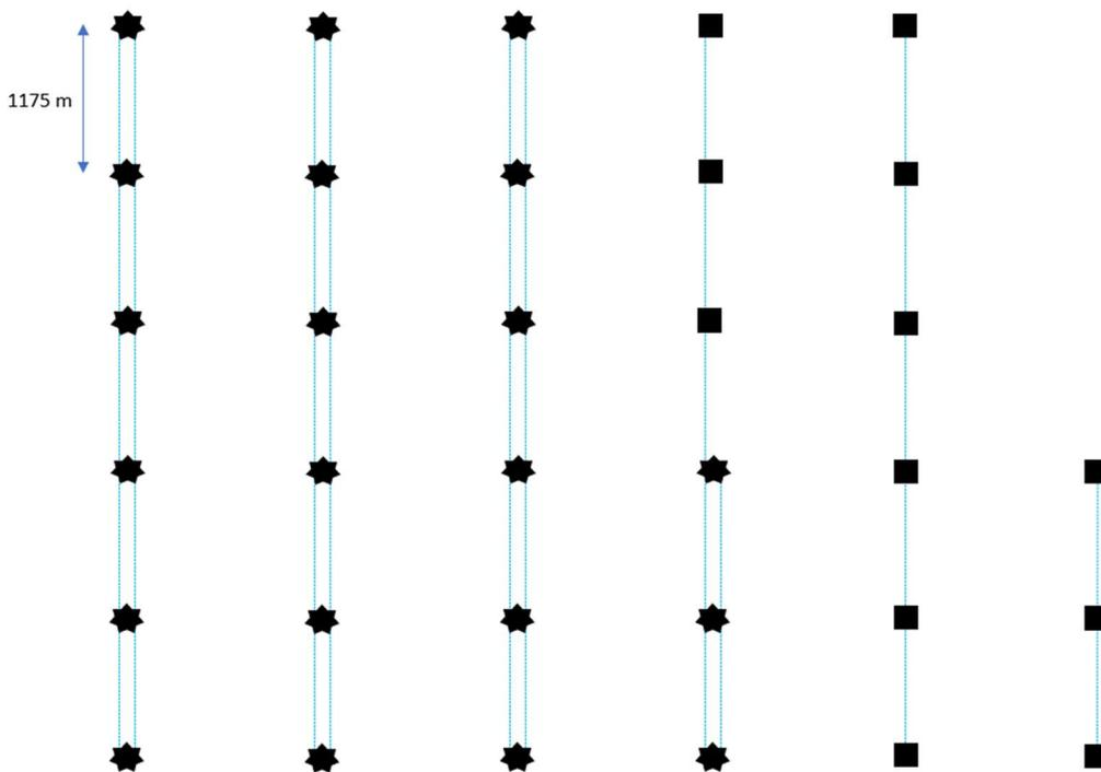
Figure 3-10: WTG and WEC layout (Scenario 15)
