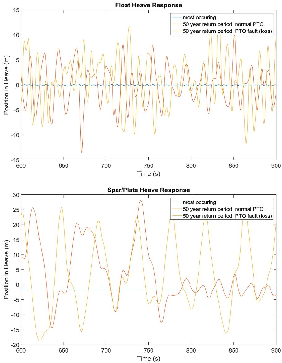
Figure 22 Extract of the float (top) and spar/plate (bottom) heave motion responses for the most occurring sea state (blue) and the 50-year return period wave under normal and loss of PTO conditions (red and orange respectively)
