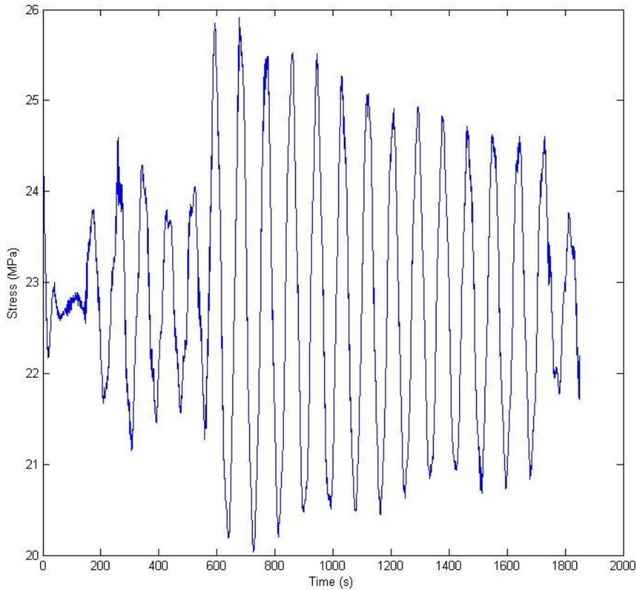
Figure 32 Stress time history for mooring line 1 for operational sea state ( $H_s = 0.75$ m and  $T_p = 5.8$ s)
