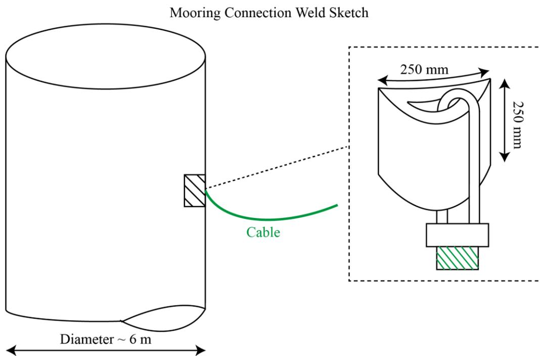
Figure 31 Assumed geometry of mooring cable to spar connection
