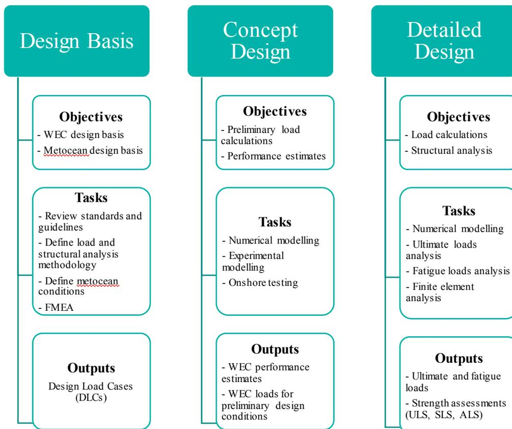
Figure 1 Key objectives and tasks: WEC design process
