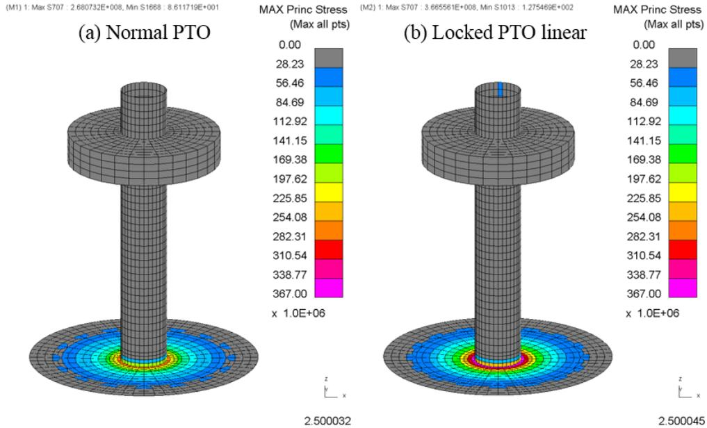
Figure 38 FEA results, maximum principal stress (max of all integration points) for (a) Normal PTO operation in extreme sea state and (b) locked PTO with loads based on linear hydrodynamics in extreme sea state
