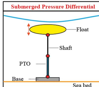
Figure 17 Schematic of example submerged pressure differential converter
