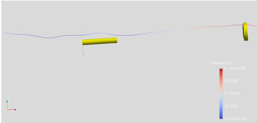
Figure 25 Snapshot of the spar/plate and float positions at  $t=380s$  under the 50-year return period wave with loss of PTO (loss of structural integrity).
