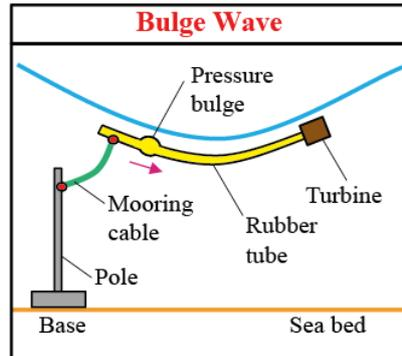
Figure 14 Schematic of example bulge wave converter
