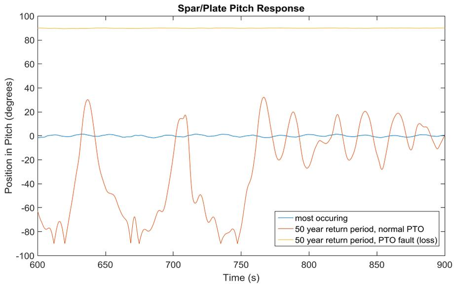
Figure 24 Extract of the spar/plate pitch motion responses for the most occurring sea state (blue) and the 50-year return period wave under normal and loss of PTO conditions (red and orange respectively)
