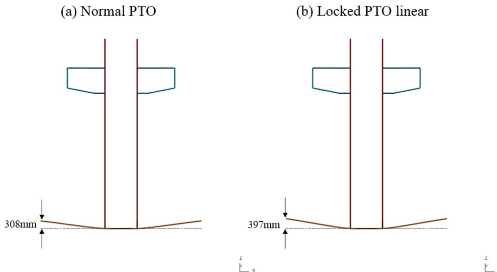
Figure 37 Cut Section of model showing base plate deformation (magnified by 5 times) after load application assuming (a) normal PTO and (b) locked PTO (linear) operation
