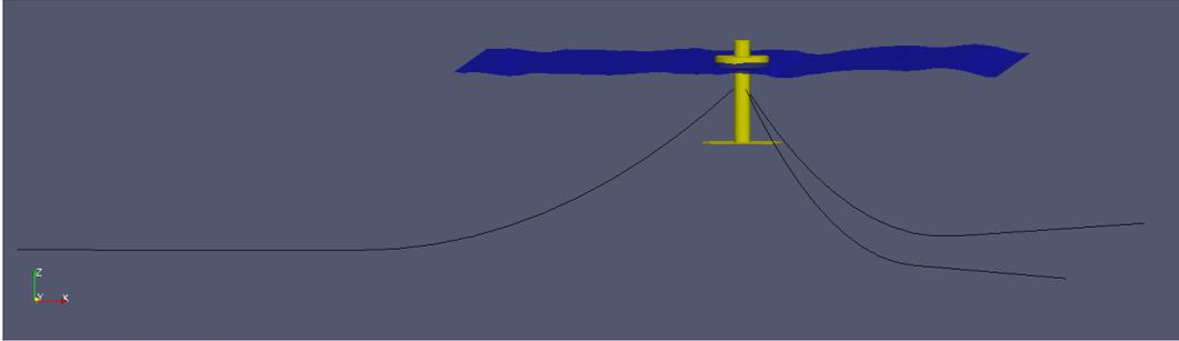
Figure 20 Mooring line arrangement schematic
