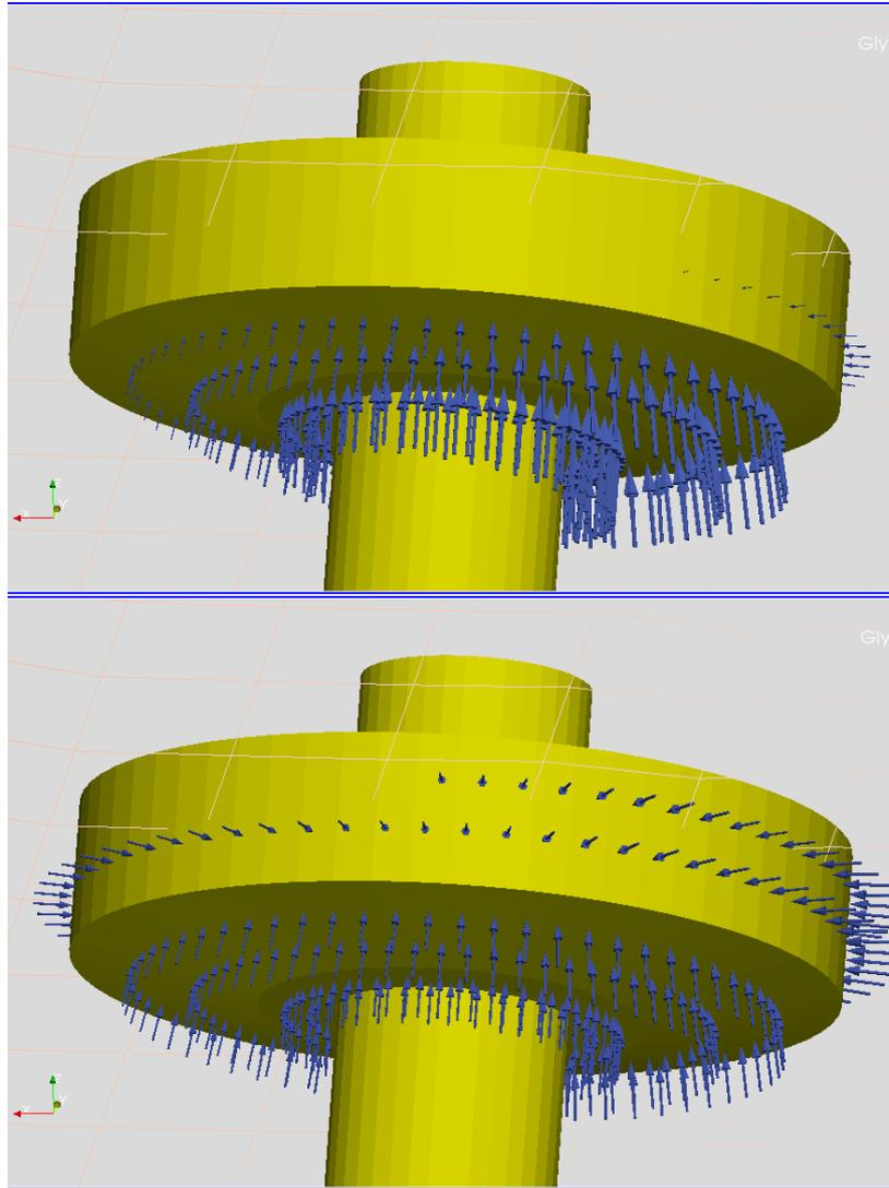
Figure 30 Distribution of pressure on the float for hydrostatic (top) and nonlinear Froude-Krylov (bottom) at  $t=811$  s ( $H_s=14.7$  m and  $T_p=18.2$  s) – normal PTO settings.
