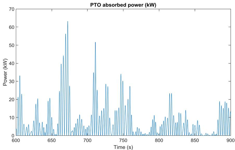
Figure 29 Extract of the absorbed power time series (kW) in the most frequently occurring sea state – 30min averaged absorbed power: 8.6kW
