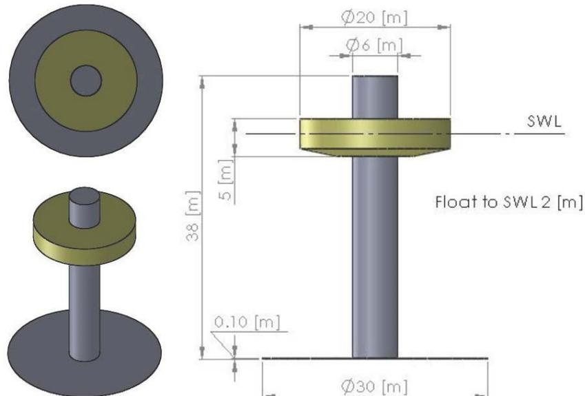
Figure 18 Dimensions of the RM3 WEC-Sim
