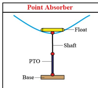
Figure 11 Schematic of an example point absorber converter
