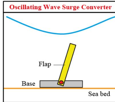
Figure 12 Schematic of an example oscillating wave surge converter
