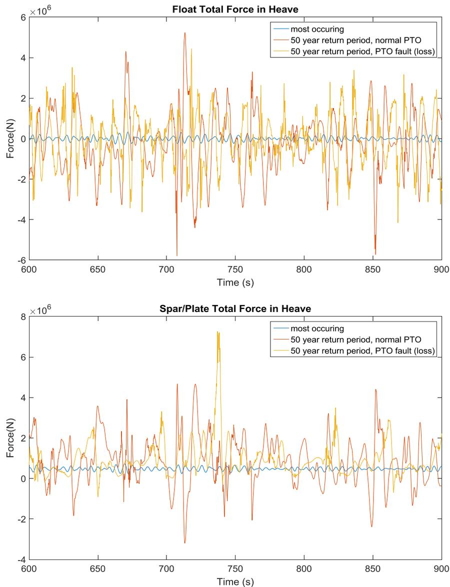
Figure 26 Extract of the float (top) and spar/plate (bottom) total heave force responses for the most occurring sea state (blue) and the 50-year return period wave under normal and loss of PTO conditions (red and orange respectively)
