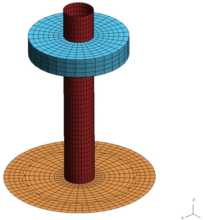
Figure 35 Shell model of point absorber analysed in LS-DYNA, consisting of 3 main components, float (blue), spar (red) and base plate (orange).
