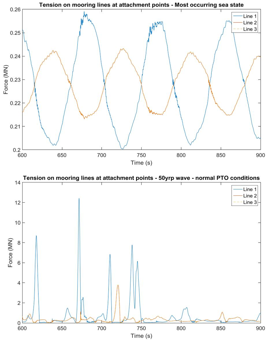
Figure 27 Extract of the tensions (in MN) on the mooring lines for the most occurring sea state (top,) and the 50-year return period wave under normal PTO conditions (bottom)
