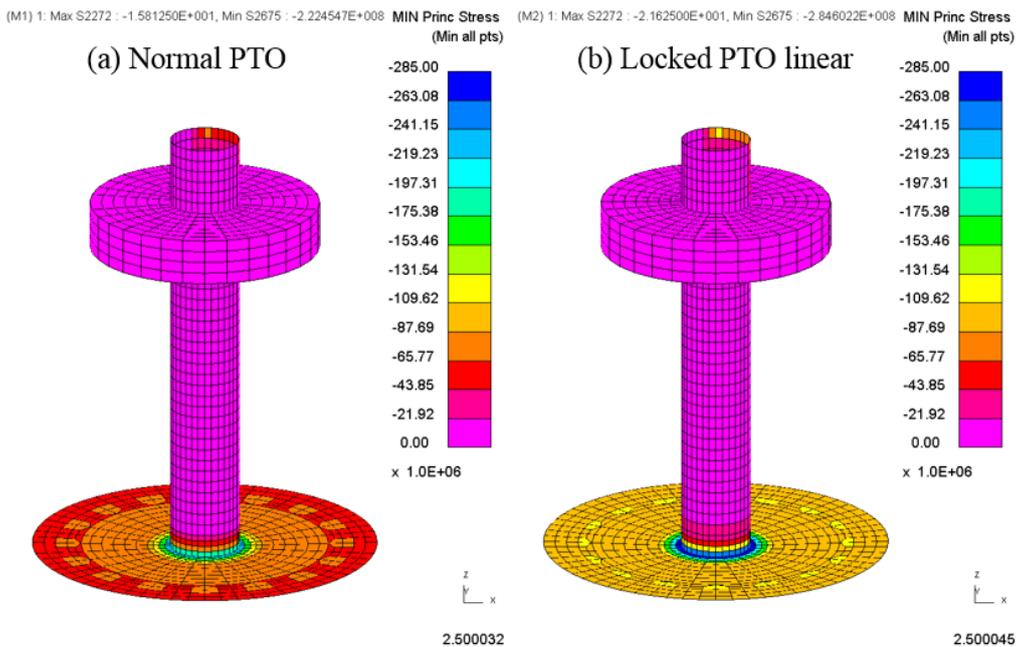
Figure 39 FEA results, minimum principal stress (minimum of all integration points) for (a) Normal PTO operation in extreme sea state and (b) locked PTO with loads based on linear hydrodynamics in extreme sea state
