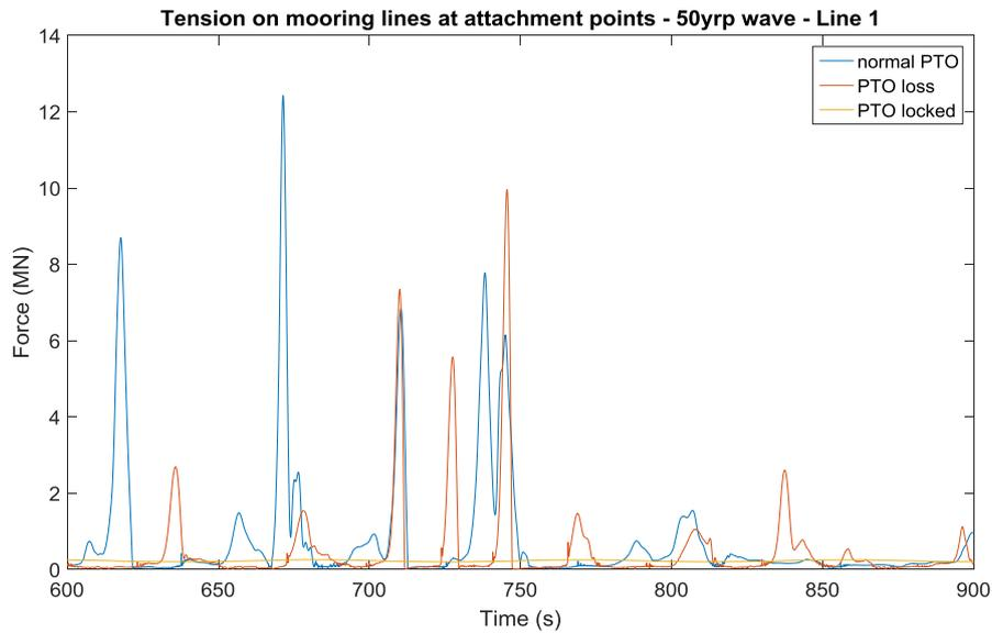
Figure 28 Extract of the tensions (in MN) on the mooring lines for the 50-year return period wave under normal PTO conditions (blue), loss of PTO (red) and lock PTO (orange)
