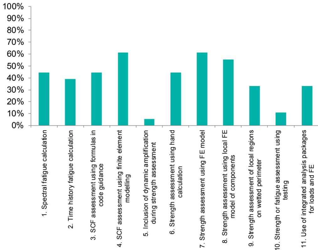
Figure 8 Methods used by respondents in the assessment of structural integrity
