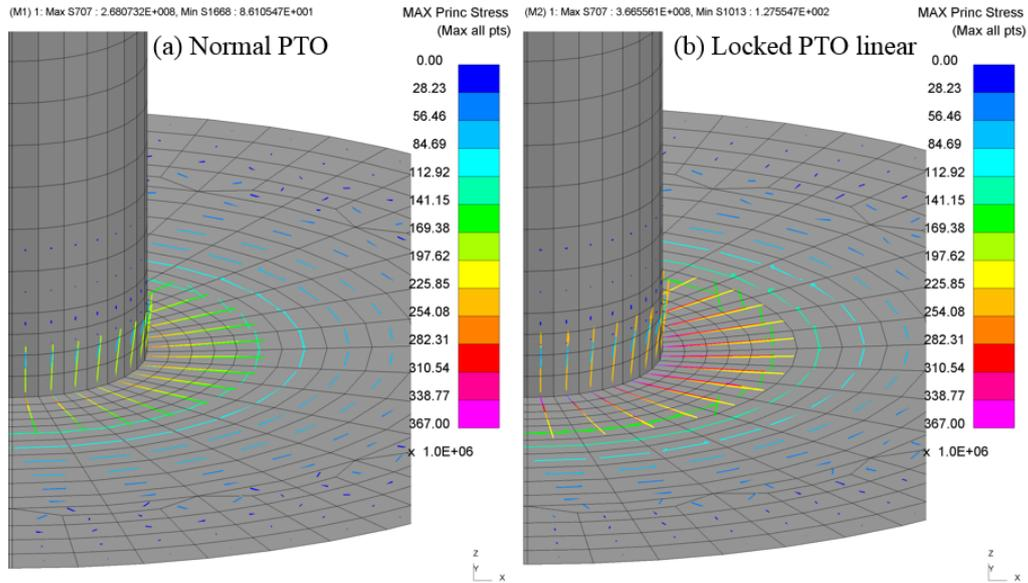
Figure 40 FEA results, maximum principal stress shown as a vector plot (max of all integration points) for (a) Normal PTO operation in extreme sea state and (b) locked PTO with loads based on linear hydrodynamics in extreme sea state
