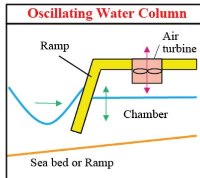
Figure 13 Schematic of example oscillating water column converter
