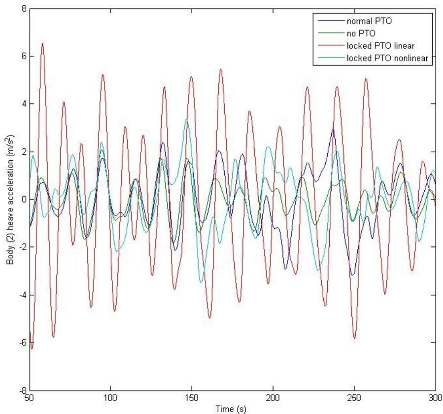
Figure 36 Acceleration time history for combined rigid body of plate and spar
