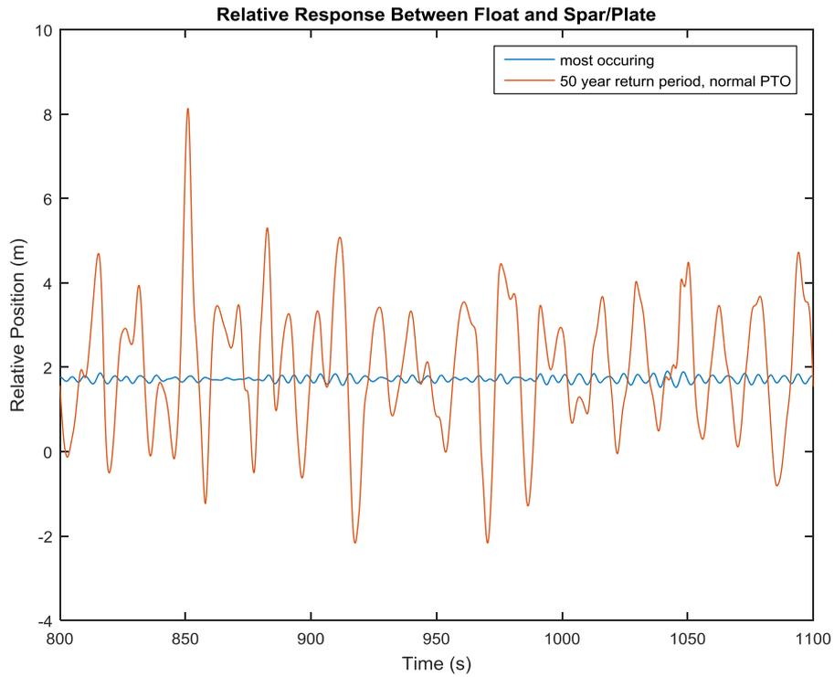
Figure 23 Extract of the relative heave motion responses between the two bodies (float and spar/plate) for the most occurring sea state (blue) and the 50-year return period wave under normal PTO conditions (red)
