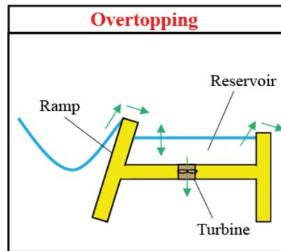
Figure 16 Schematic of example overtopping converter
