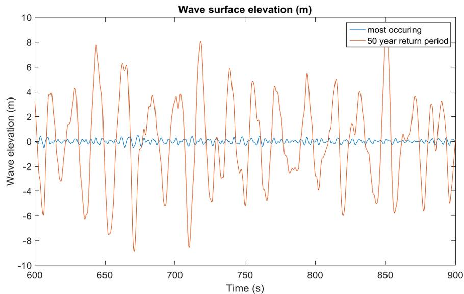
Figure 21 Extract of the wave surface elevation time-series for the most occurring sea state (blue) and the 50-year return period wave (red)
