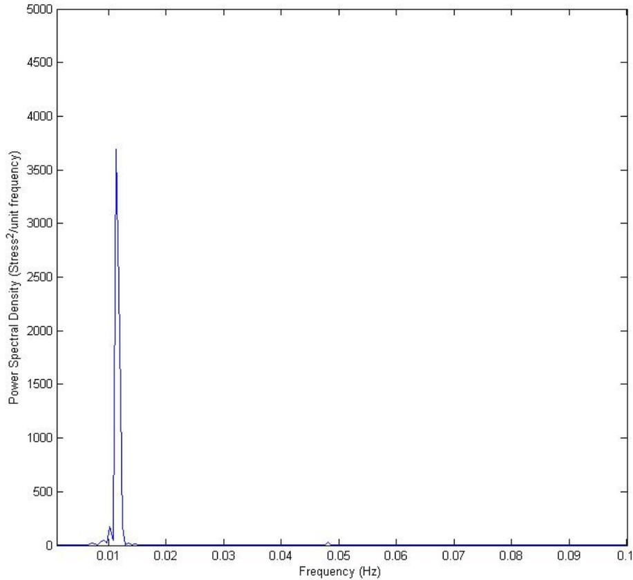
Figure 33 Power spectral density plot (frequency domain) for mooring line 1 for an operational sea state with 0.75m significant wave height and 5.8s peak period
