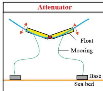
Figure 15 Schematic of example attenuator converter
