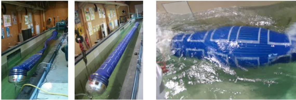
Figure 4-13. SBM S3 bulge wave WEC during wave tank testing, reproduced from SBM Offshore [191].
